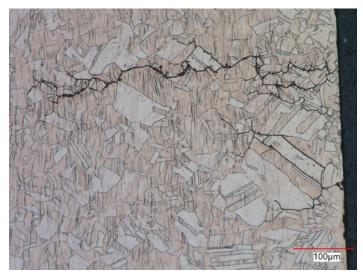
Above: Microstructure of a metallographic sample from copper pipe showing secondary branched cracks, typical for stress corrosion cracking degradation mechanism.
