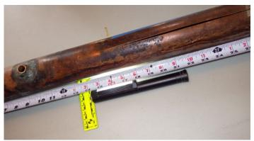
Above: Copper riser that was bent in service and which developed a longitudinal split. Stresses induced in the pipe due to bending contributed to the formation of the split.
