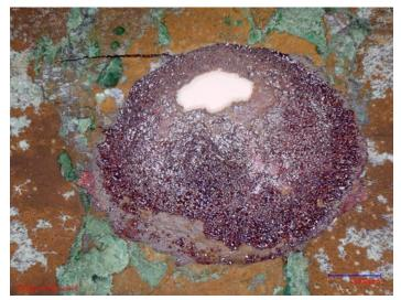
Above: Optical microscope image of pitting on the internal surface and wall perforation of a copper pipe due to addition of undesirable chemicals in chlorinated water (magnification x50).
