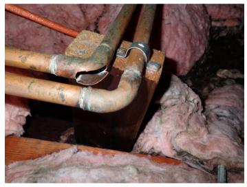
Above: Split with fish mouth appearance in a 900 copper elbow which was typical for failure due to freezing. The piping was installed in non-heated attic space and it was not protected from freezing.
