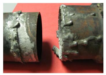
Above: Substandard soldered joint exhibiting improper surface preparation and excessive solder beading.
