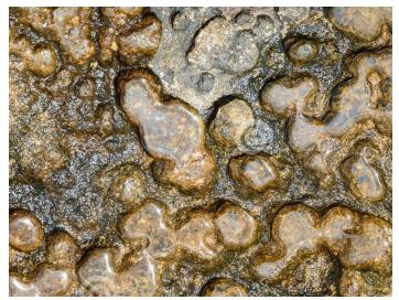
Above: Stereo microscope image of the inner surface of a copper tube affected by erosion-corrosion. Scooped appearance in areas where the pipe material was eroded and swept away.
