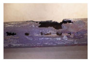
Above: Copper piping that failed as the result of stray current corrosion because of improper grounding of electrical appliances.
