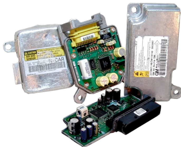
Figure 1: View of an airbag control module from a passenger vehicle. This module's secondary function is an event data recorder (EDR) to capture collision related information.
